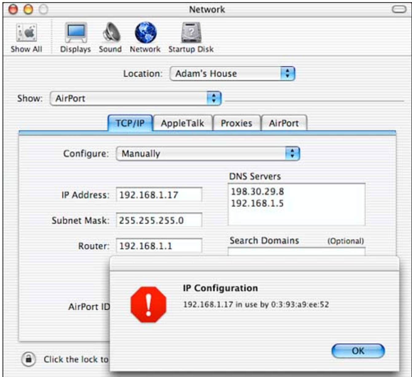
Figure 8.2. Macs check for other machines on the network with the same IP address they're trying to claim when they try to initialize their network interfaces.
