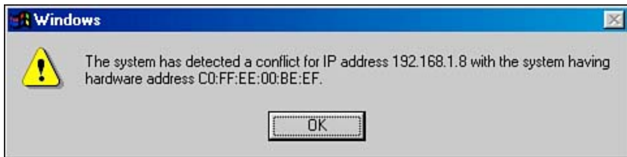
Figure 8.3. Wintel boxes check when the network interface is initialized, but also pop up annoying conflict dialogs whenever any other machine tries to register a duplicate IP at a later time.
