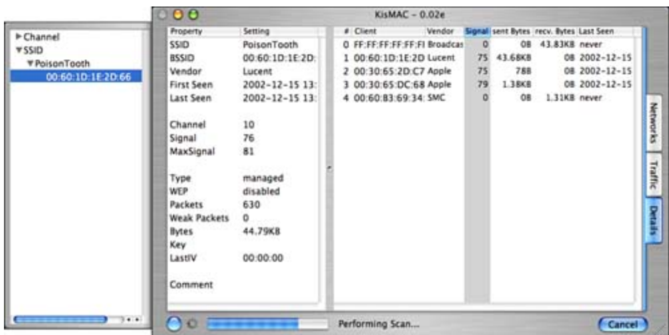
Figure 7.6. KisMAC can sniff out wireless networks and even crack WEP encryption.
